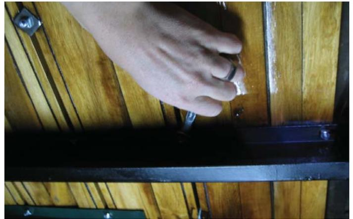
was the built-in square on the bolt pushing against the square cutout hole on the metal strips. If you were to over-tighten the nut, these square cutout holes would be the first to fail. Don't ask me how I know this. ☺
