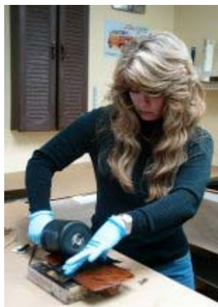
Using a urethane roller to transfer the pattern
