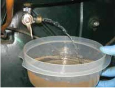
Unable to move under its own power, I pushed the Model A out of the garage and into the driveway. I turned off the fuel and drained the lines. Removing the internal lines was easy. I ran a thin long wire through each section of fuel line. No debris
