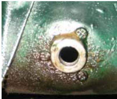
ran another five bowls through the tank, just to make sure. I then taped a shop towel onto a long screwdriver and ran it down through the gas filler along the bottom and sides of the tank to see what would appear on the light blue shop towel. As you can see by the pictures, not much solid debris remained. Finally I strained the bits of debris out of the five gallons of gas.
