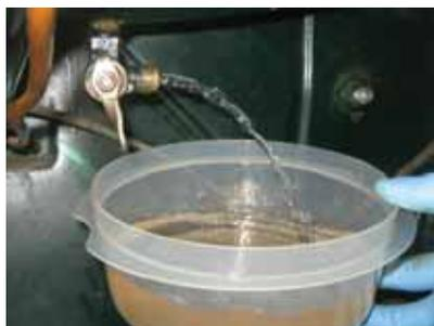
Unable to move under its own power, I pushed the Model A out of the garage and into the driveway. I turned off the fuel and drained the lines. Removing the internal lines was easy. I ran a thin long wire through each section of fuel line. No debris
