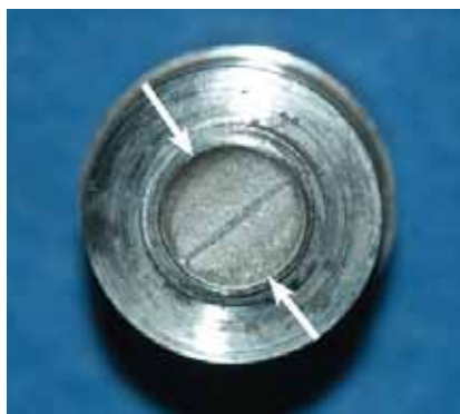
Photograph B: Fracture surface from a large electronic gate pivot pin. The white arrows indicate the fatigue crack origin.
