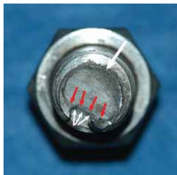
Photograph C1: Two way bending fatigue in a bolt. Large Arrow at 1 o'clock shows area of fatigue crack initiation.
