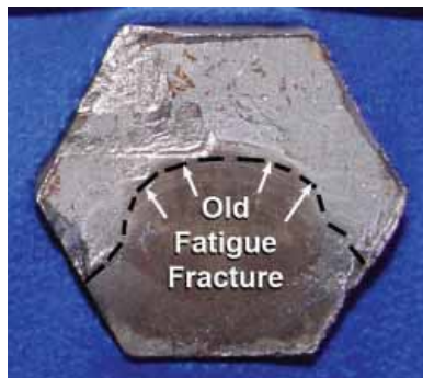
Photograph C2: Overall view of fatigue failure on hexagonal shaped jackhammer tool.
