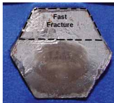
Photograph C4: Final fast fracture region of fatigue crack was created at the final instant of failure and separation.
