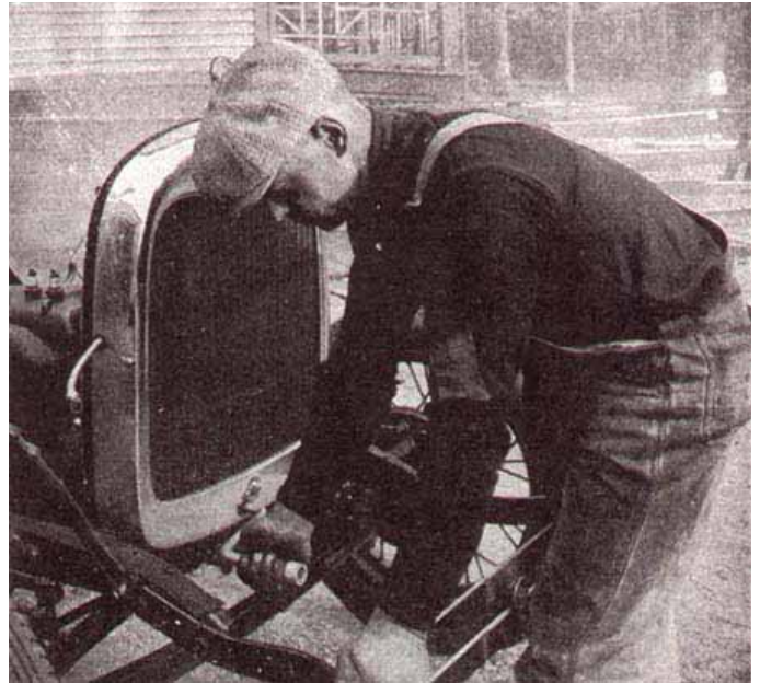
Always grip the crank with the thumb wrapped below with the fingers NEVER push the crank down the right side of the rotation!
